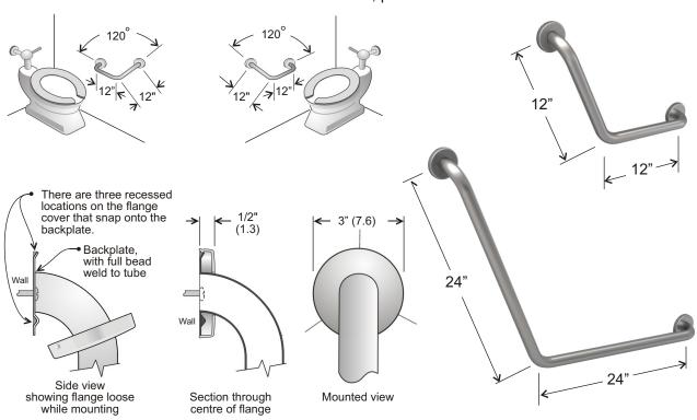
Concealed mounting screws, using snap flange, on "SP & NP" codes
