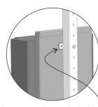
When mounting code 2010 to standard perforated tubing "sandwich bolt plate between 2011 liner holder and perforated tubing. Use centre rectangular hole.
