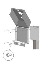
Use 10-24 machine screws when mounting the Code 2010 to the Code 909-100 Stand.
