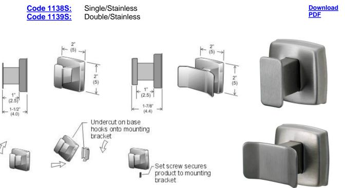
**Mounting of Product:** Screw concealed mounting system: The mounting bracket is attached to the wall with screws at the desired height. The unit is then hooked onto the bracket. When the set screw is tightened the product is firmly secured to the wall. The set screw applies pressure to an inclined surface on the bracket this provides a rattle free and integral mounting of the product. (mounting bracket and screws provided).
